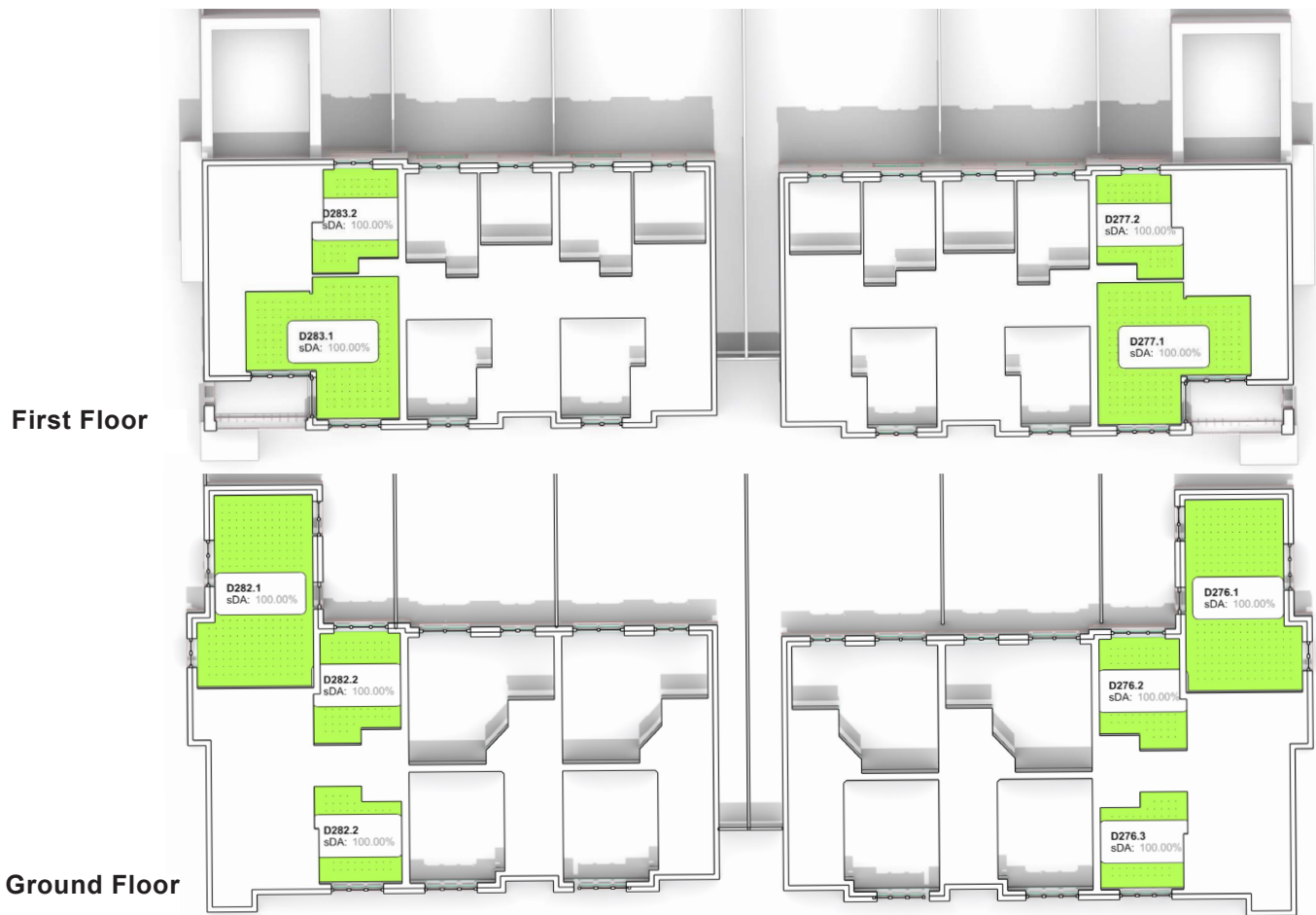
Figure 39: Duplex units 276 - 277 and 282 - 283 Daylight Provision BS EN17037:2018+A1:2021 Table NA.1 compliance for all habitable rooms
