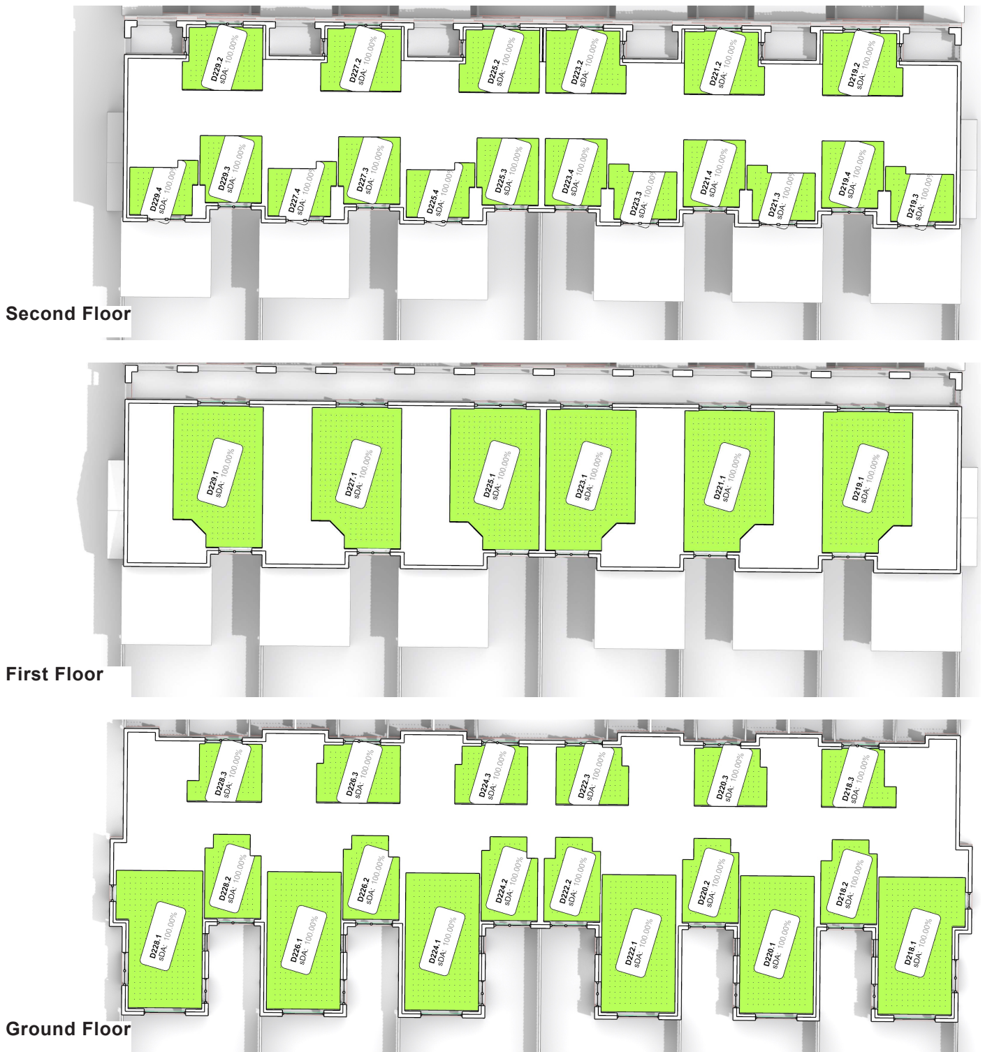
Figure 36: Duplex units 218 - 229 Daylight Provision BS EN17037:2018+A1:2021 Table NA.1 compliance for all habitable rooms
