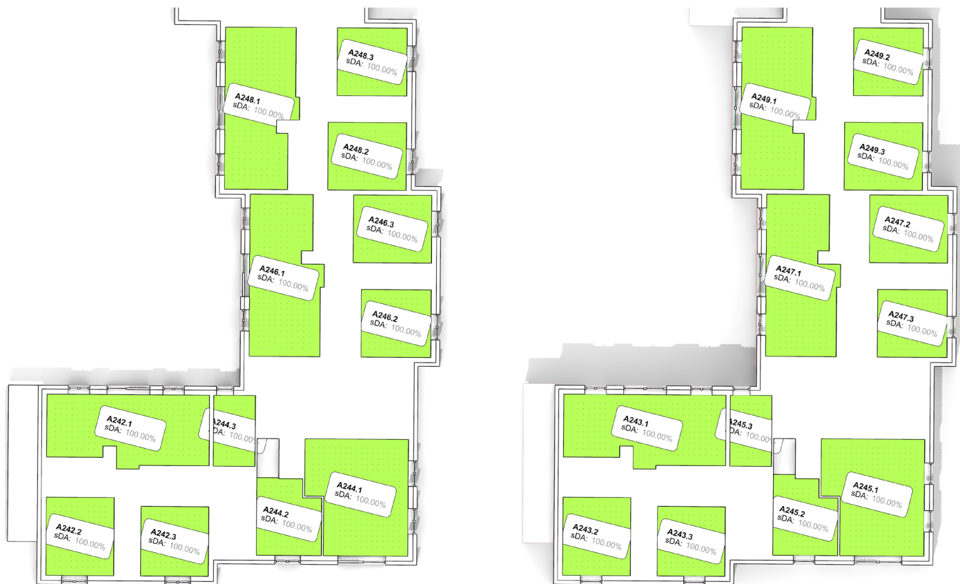
Figure 29: Apartment Block C - Daylight Provision BS EN17037:2018+A1:2021 Table NA.1 compliance for all habitable rooms
