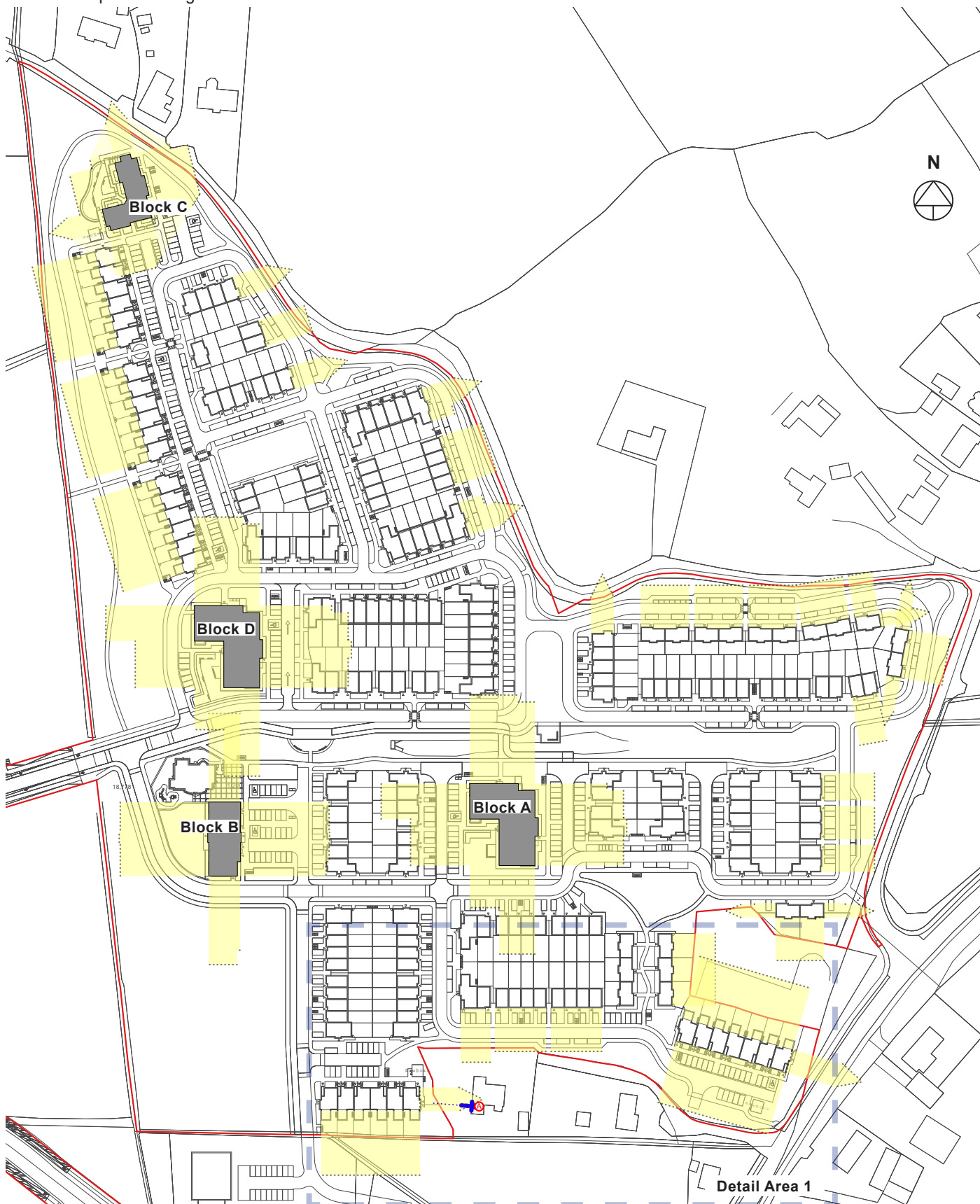
Figure 2: Proposed site plan showing the zone of influence (3 times the height of the proposed building) and direction of the window wall of adjacent residential properties.
