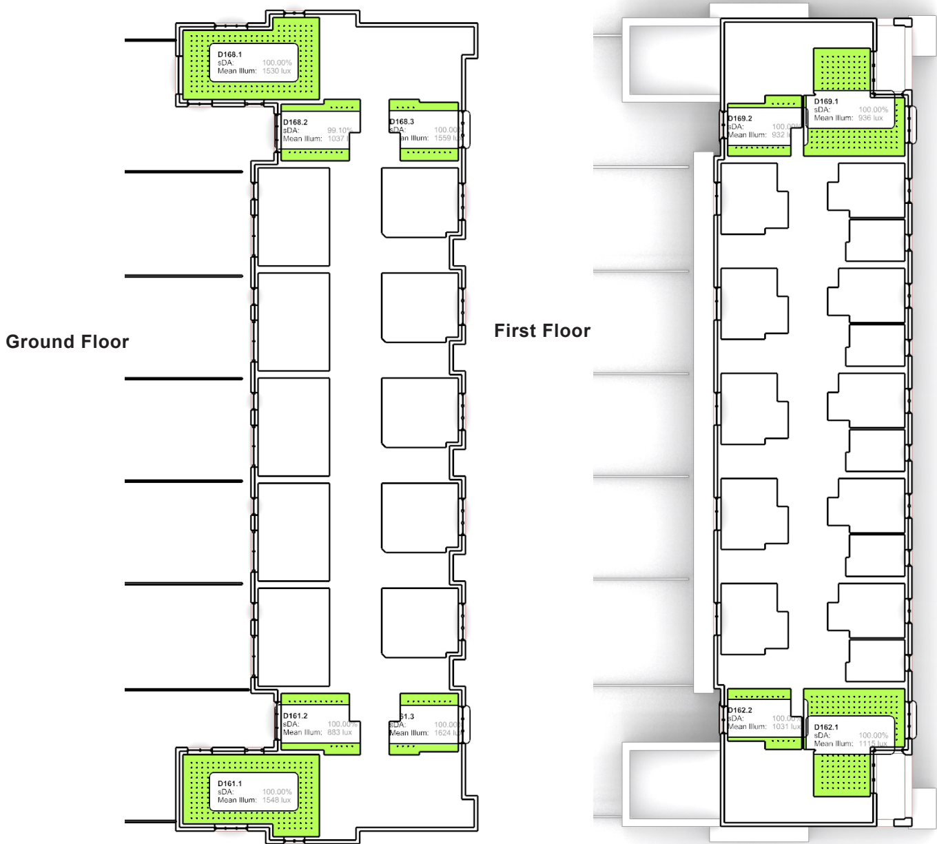
Figure 34: Duplex units 161 - 162 and 168 - 169 Daylight Provision BS EN17037:2018+A1:2021 Table NA.1 compliance for all habitable rooms
